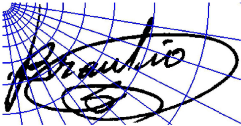
Fig. 4. Log-polar grids, origin taken as the top-left corner.
