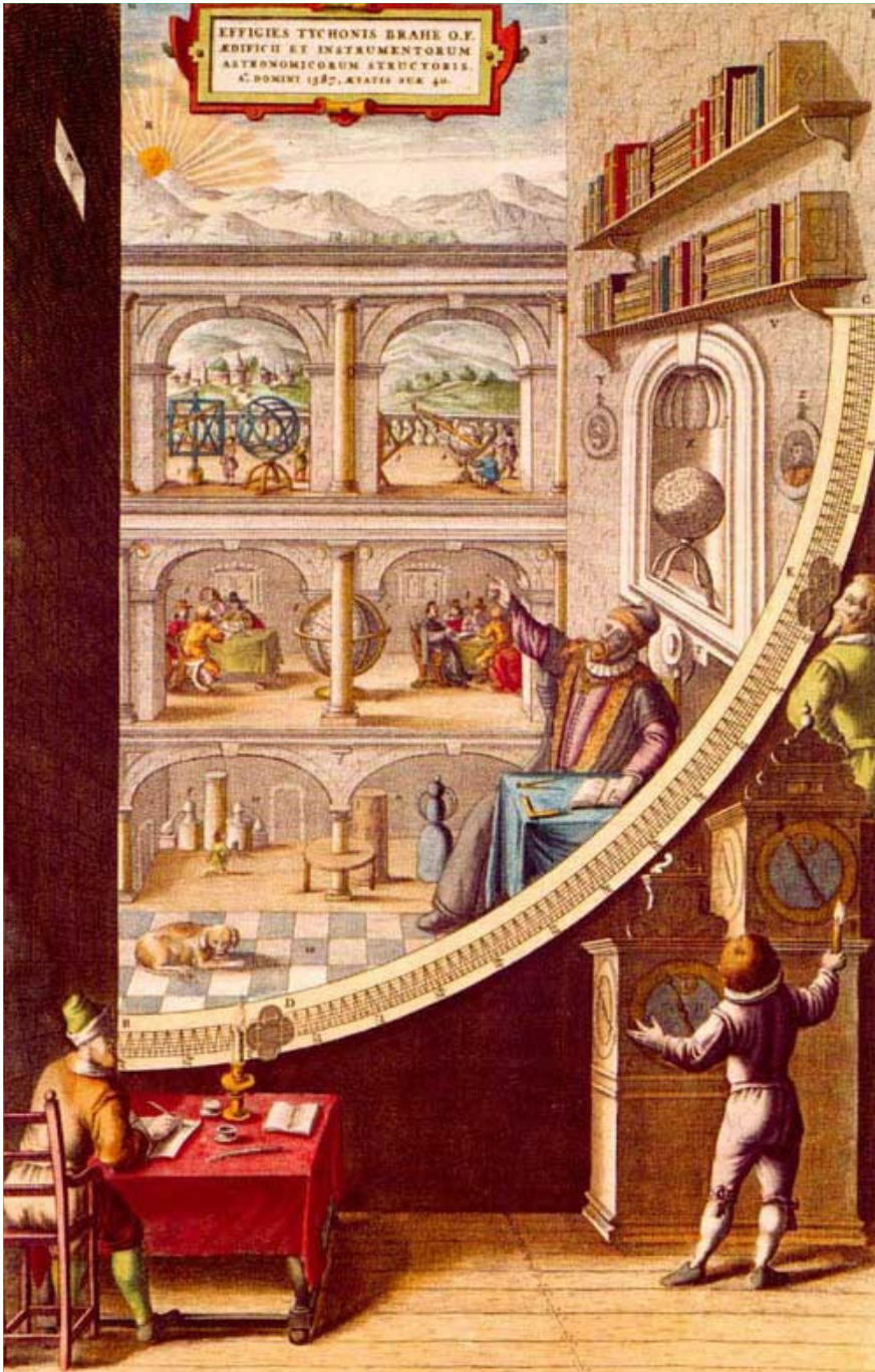
The great Wall Quadrant. Copper etching from Blaeu's Atlas Major, 1663. Made following a depiction in Tycho Brahe's Astronomiae Instauratae Mechanica.
