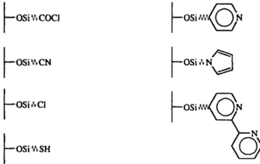
Figure 6.3 Some examples of functional groups which have been attached to surfaces by use of the corresponding reactive organosilanes. \sim represents a generalized linking chemical group such as an alkyl chain.
