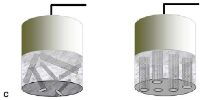
Figure 3. Three configurations of CNT integration in electrochemical sensors. (A) Use of individual CNT: for AFM tips (left) or individual SWCNT onto a Si wafer substrate (right). SiOx and PMMA are used as insulating layers in which windows are opened to expose the SWCNT; (B) electrode surface modifiers: non-oriented (left) and oriented (right) CNT configuration; and, (C) composites with non-oriented (left) and oriented (right) CNT configuration.
