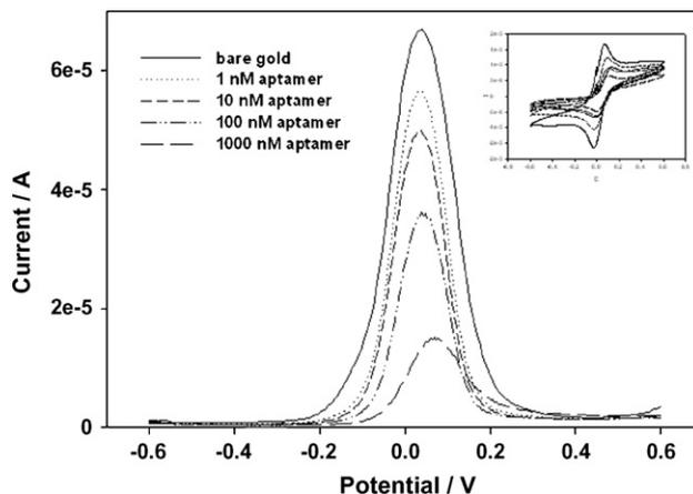
**Fig. 3.** Electrochemical analysis for immobilization of thiol-modified aptamer on IDA gold electrode. The current was decreased depending on the concentration of ssDNA aptamer in square wave voltammogram. The inset figure shows cyclic voltammogram.
