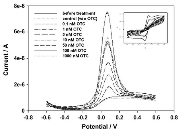
**Fig. 4.** Electrochemical analysis of OTC using aptamer-immobilized IDA gold electrode: The current drop was proportional to the concentration of OTC in a range 1–100 nM from square wave voltammogram. The inset figure shows cyclic voltammogram.
