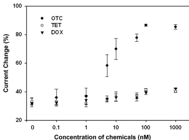
**Fig. 5.** Quantitative and specific detection of OTC. Electrochemical analysis was conducted by applying a series of OTC, TET and DOX concentrations (0.1, 1, 5, 10, 50, 100, 1000 nM) on aptamer-immobilized IDA gold electrode chip.
