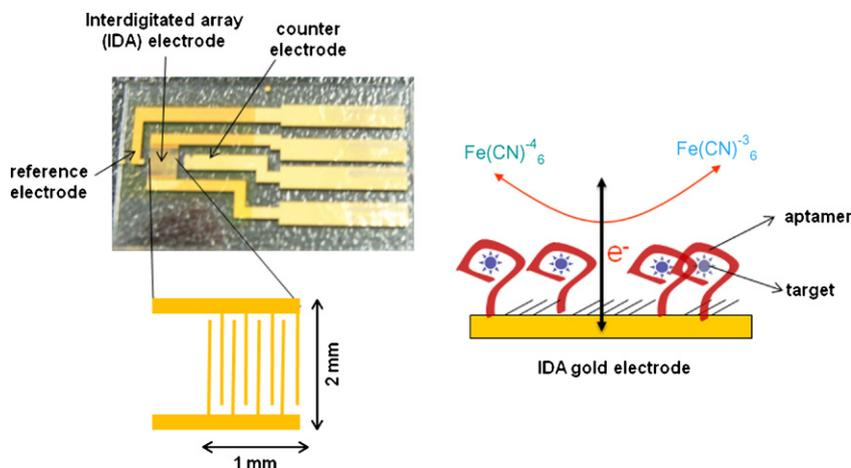
**Fig. 2.** Schematic diagram of electrochemical detection system for oxytetracycline (OTC) using aptamer-immobilized inter digitated array (IDA) gold electrode chip. (A) A photograph of an IDA gold electrode chip, (B) schematic diagram of IDA gold electrode showing magnified region of IDA, and (C) schematic diagram of a typical electrochemical reaction occurring after aptamer binds to its target molecule on a gold IDA electrode chip.
