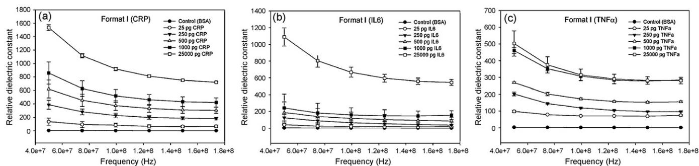
**Fig. 2.** Changes in dielectric responses to different concentration of pure protein biomarker targets: (a) CRP; (b) IL6, and (c) TNF $\alpha$  as a function of frequency in format I in which each capacitor array contained anti-CRP, anti-IL6, and anti-TNF $\alpha$ , respectively.
