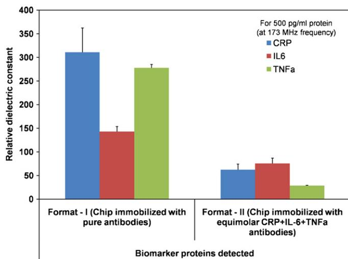
**Fig. 3.** Changes in dielectric response against 500 pg/ml concentration of protein biomarker targets (CRP, IL6, and TNF $\alpha$ ) at a frequency of 173 MHz. The biomarkers are allowed to incubate sequentially on GID-capacitor arrays immobilized with antibodies (anti-CRP, -IL6, and -TNF $\alpha$ ) in pure form (format I) and in mixture (1:1:1) multiple, respectively. The number of binding sites in format II contains three times lesser than that in format I.
