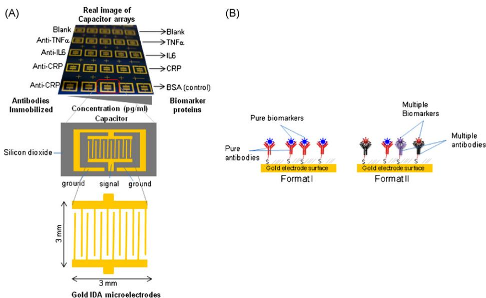
**Fig. 1.** Schematic representation of (a) GID-capacitor array chip and (b) GID region of each capacitor immobilized with pure (format I) and multiple antibodies (format II) and capturing of protein biomarker target/s.
