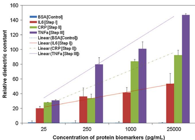
**Fig. 4.** Multiplexed detection of protein biomarkers on chips immobilized with equimolar mixture of anti-CRP, -IL6 and -TNF $\alpha$  antibodies (format II) and the concentration dependent increase in dielectric response within 173 MHz frequency are shown in the figure. The coloured lines shown are derived of linear fit for corresponding values for tested biomarker proteins and BSA protein was used as a negative control.
