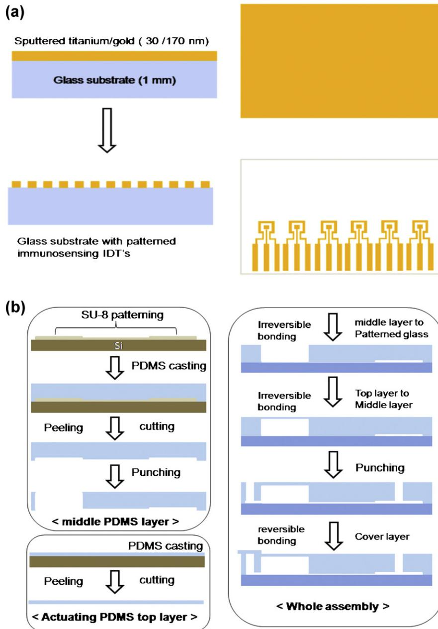
**Fig. 2.** (a) Fabrication process flow of inter-digitated transducers on glass substrate. (b) Fabrication process flow for the PDMS-based immunosensing LOC with pre-patterned glass as substrate.
