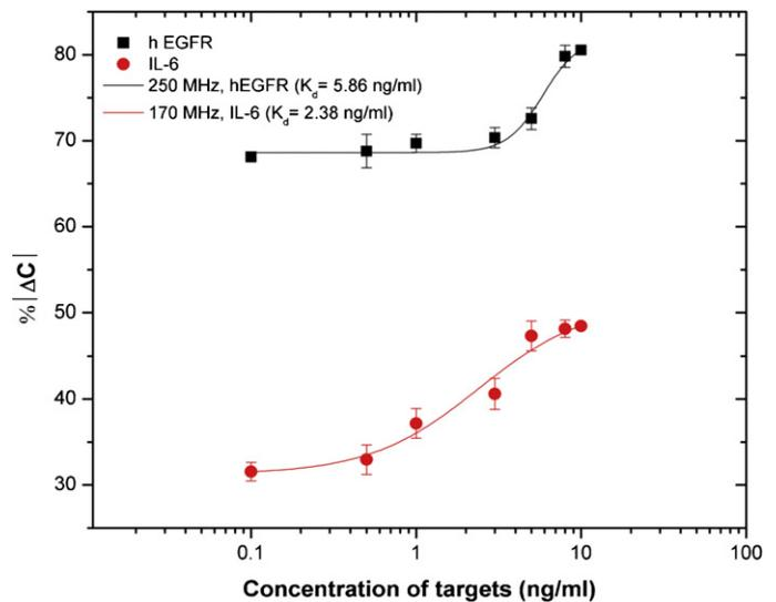
**Fig. 6.** Dose-dependent change in relative capacitance occurred after the Ab–Ag complex formation on IDT surface against varying concentrations of hEGFR at 270 MHz and IL-6 target in serum (0.1–10 ng/ml) at 170 MHz frequency.
