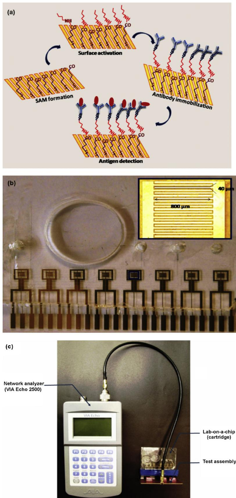
**Fig. 4.** (a) Schematic diagram of the bio-functionalization of the IDT surface. (b) Photographic image of the LOC system. (c) Hand-held format of measurement system.
