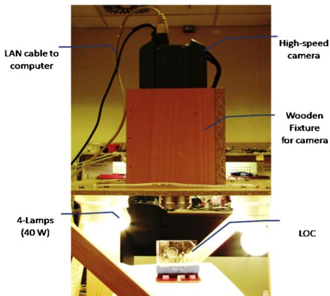
**Fig. 3.** Photographic representation of the experimental setup used for the flow characterization.
