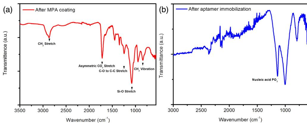
**Fig. 1.** Changes in FTIR spectra after capacitor chips subjected to; (a) self-assembled monolayer formation with MPA and (b) covalent coupling of anti-HER2 ssDNA aptamers.
