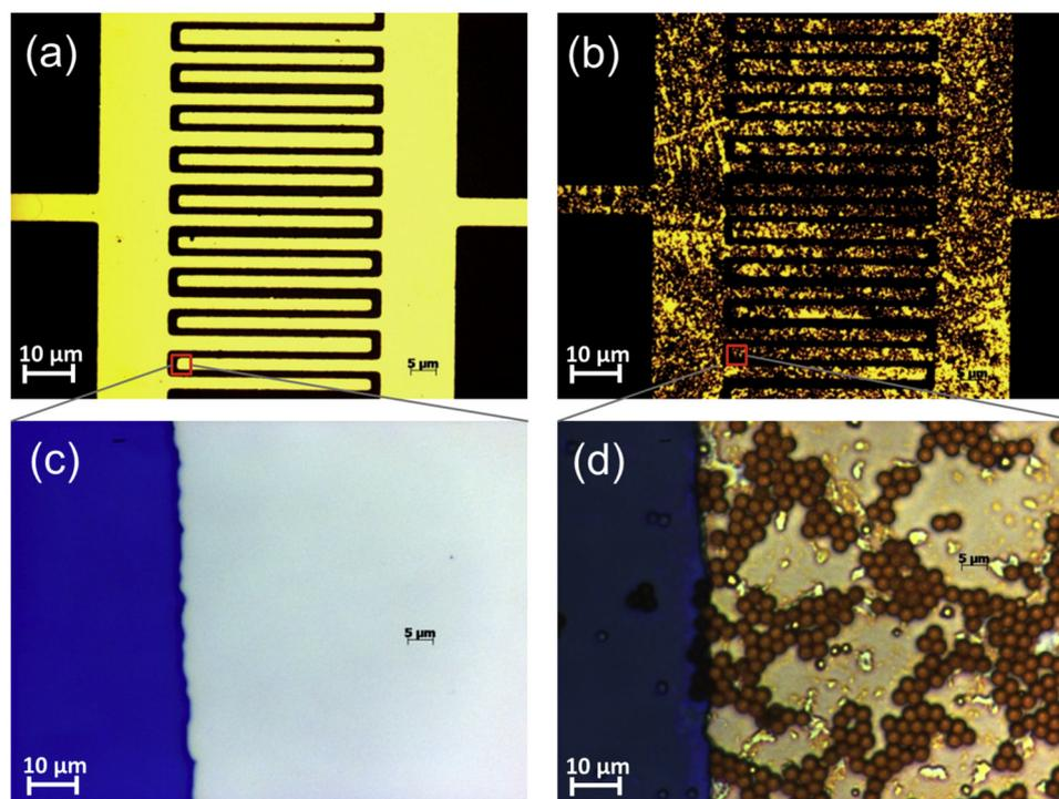
**Fig. 2.** Optical microscopic images of sensor surface: (a) control and (b) after sandwiching with MB-Abs (magnetic beads functionalized with VEGF antibodies). Images shown in (c) and (d) are enlarged view of a portion from (a) and (b), respectively that were taken at higher resolutions (100 $\times$ ).
