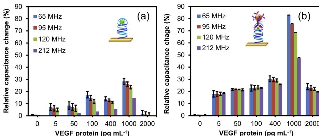
**Fig. 4.** Relative percent changes in capacitance responses occurred at different frequencies (65, 95, 120 and 212 MHz) with: (a) primary complex (aptasensor, before sandwiching) and (b) secondary complex (apta-immunosensor, after sandwiching with MB-Abs) formed on the sensor surfaces. The insets in figures (a) and (b) represent illustrations before and after sandwiching of aptamer-VEGF protein complex with MB-Abs.
