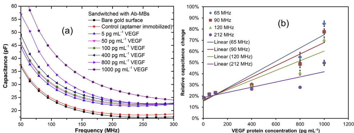
**Fig. 3.** (a) Capacitance response profiles as a function of applied AC frequency with the developed apta-immunosensor upon sandwiching with constant amounts of monoclonal antibodies for VEGF protein coated on MB-Abs on the aptamer-VEGF protein complex previously formed on the sensors. (b) Percent relative change in capacitance responses of apta-immunosensor extracted at four different frequencies indicated in figure legend and the data were fitted with linear regression analysis.
