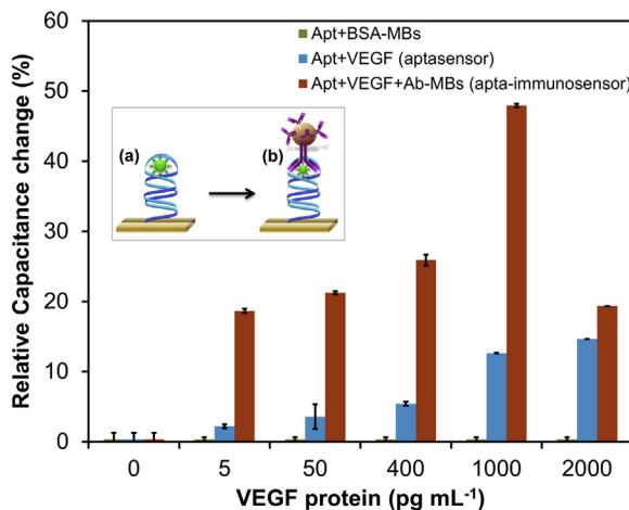
**Fig. 5.** Comparative relative percent change in capacitance responses at 212 MHz with primary complex (aptasensor) and secondary complex (apta-immunosensor) formed on sensor surfaces. The inset figures (a) and (b) illustrates the formation of complex on a section of gold IDE surface before and after the signal enhancement, respectively.
