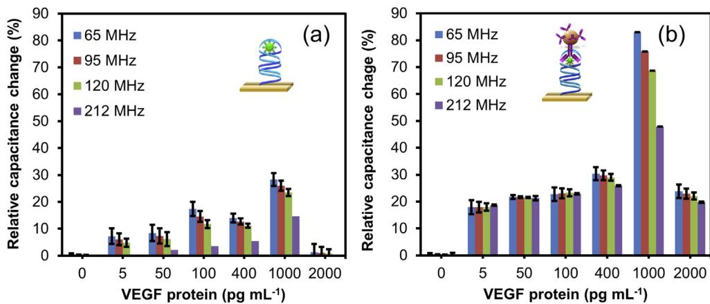
**Fig. 4.** Relative percent changes in capacitance responses occurred at different frequencies (65, 95, 120 and 212 MHz) with; (a) primary complex (aptasensor, before sandwiching) and (b) secondary complex (apta-immunosensor, after sandwiching with MB-Abs) formed on the sensor surfaces. The insets in figures (a) and (b) represents illustrations before and after sandwiching of aptamer-VEGF protein complex with MB-Abs.
