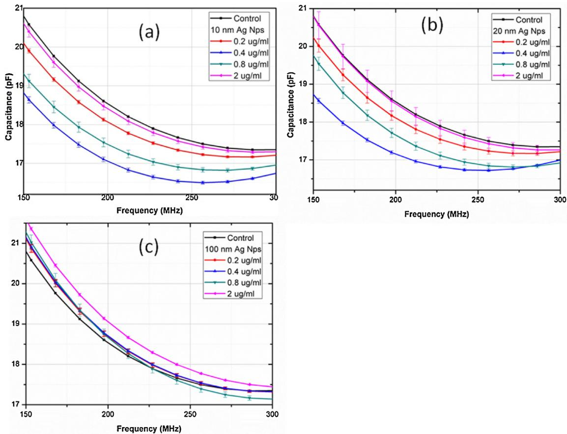
**Fig. 3.** Change in capacitance from whole-cell chip as a function of applied frequency (100–300 MHz) when exposed to different concentration (0.2–2  $\mu$ g/ml) of (a) 10 nm (b) 20 nm and (c) 100 nm size of Ag NPs.
