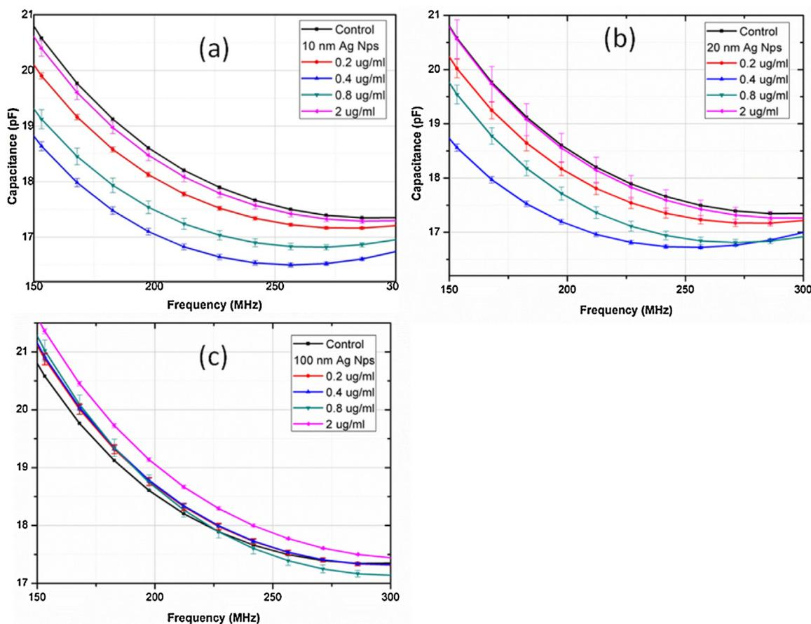
**Fig. 3.** Change in capacitance from whole-cell chip as a function of applied frequency (100–300 MHz) when exposed to different concentration (0.2–2  $\mu\text{g}/\text{ml}$ ) of (a) 10 nm (b) 20 nm and (c) 100 nm size of Ag NPs.
