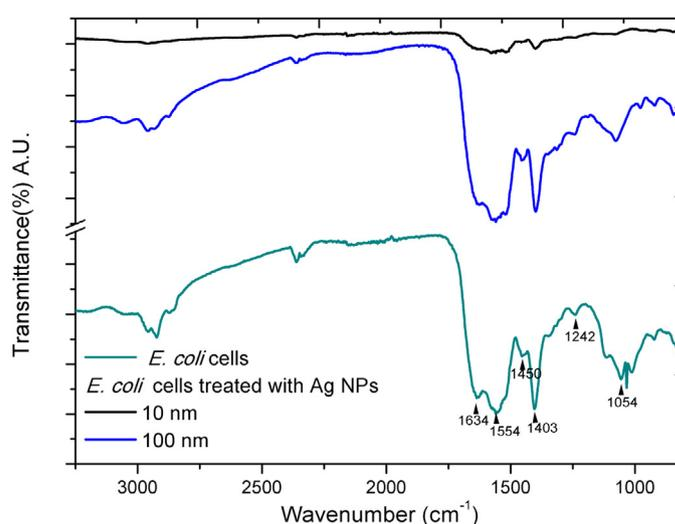
**Fig. 5.** FTIR spectra of *E. coli* cells-on-chip treated before and after exposure of Ag NPs with different sizes.
