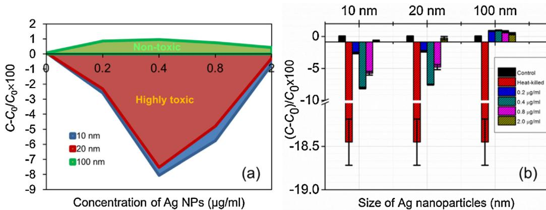
**Fig. 4.** a Relative change in capacitance responses at 200 MHz from whole-cell chip against three different sizes such as 10, 20 and 100 nm of Ag NPs at various concentrations ranging from 0.2–2 µg/ml on sensor chip. Areas under the curves are filled to distinguish effects on different sizes of Ag NPs based on the extent of toxicity effects. Fig. 4b shows bar graph of along with heat-killed cell (HKC) responses.
