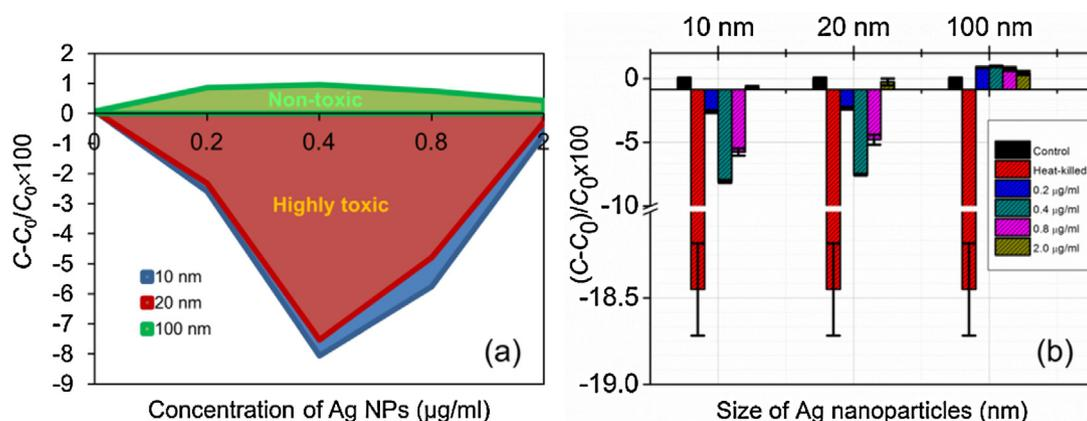
**Fig. 4.** a Relative change in capacitance responses at 200 MHz from whole-cell chip against three different sizes such as 10, 20 and 100 nm of Ag NPs at various concentrations ranging from 0.2–2  $\mu\text{g/ml}$  on sensor chip. Areas under the curves are filled to distinguish effects on different sizes of Ag NPs based on the extent of toxicity effects. Fig. 4b shows bar graph of along with heat-killed cell (HKC) responses.
