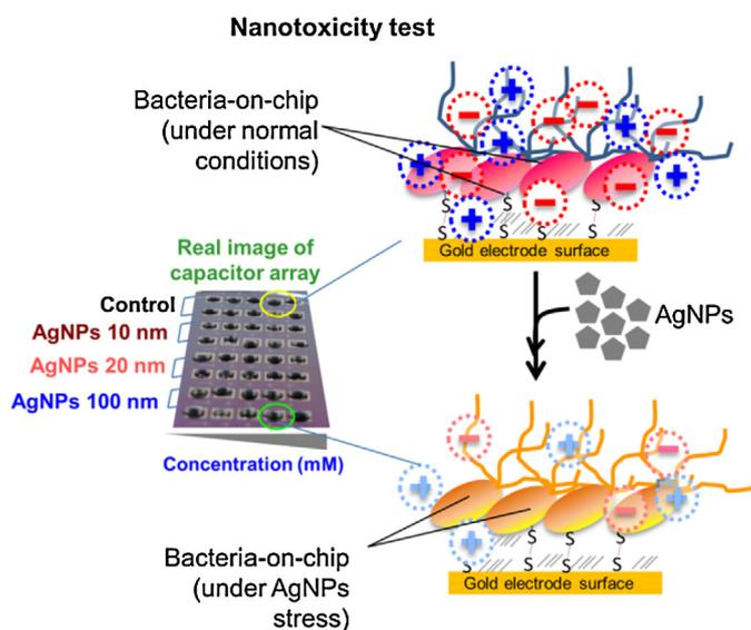
Scheme 1. Schematic of CoCT platform for probing toxicity of NPs.
