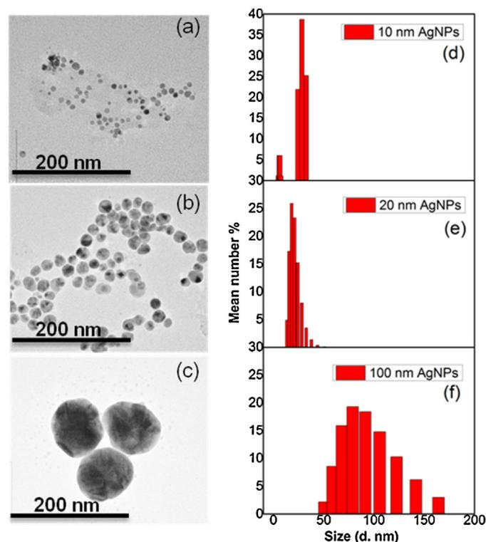
Fig. 1. (a–c) TEM images and (d–f) DLS size distribution of 5, 20 and 100 nm sizes of Ag NPs.
