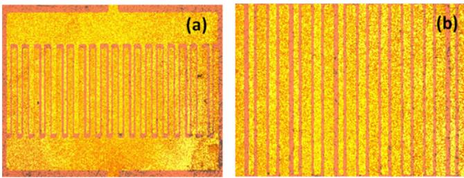
**Fig. 2.** Optical microscopic images of *E. coli* cells immobilized on; (a) capacitor chip at 5 $\times$  and (b) a magnified portion of interdigitated electrodes of capacitor chip at 10 $\times$  magnification.
