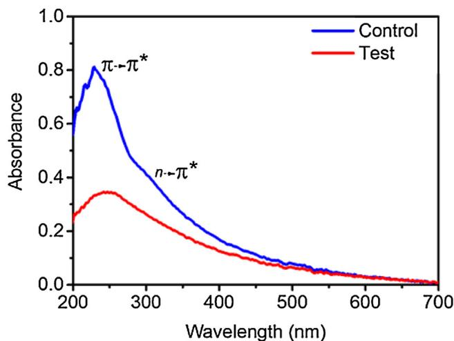
**Fig. 3.** UV-vis spectra of GO samples extracted from control culture medium (without bacteria) and test culture medium (with resistant bacteria). Control GO exhibited two absorption peaks at 230 and ~300 nm that corresponds to the  $\pi$ - $\pi^*$  transition of the C–C bonds and  $n \rightarrow \pi^*$  transition of the C=O bonds, respectively. The plasmon peak shift in test GO at 250 nm is attributed to possible reduction of GO due to biocatalytic action of nanomaterial resistant bacteria.
