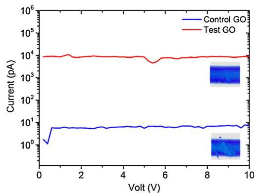
**Fig. 5.** Current-voltage characteristics of GO samples extracted from control culture medium (without bacteria) and test culture medium (in presence of resistant bacteria). The inset images show respective GO nanosheets casted between the gold electrodes.
