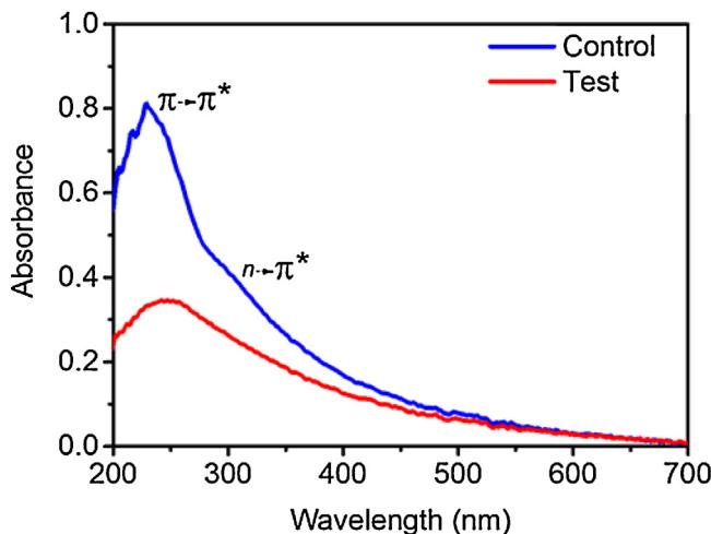
**Fig. 3.** UV-vis spectra of GO samples extracted from control culture medium (without bacteria) and test culture medium (with resistant bacteria). Control GO exhibited two absorption peaks at 230 and  $\sim$ 300 nm that corresponds to the  $\pi-\pi^*$  transition of the C=C bonds and  $n-\pi^*$  transition of the C=O bonds, respectively. The plasmon peak shift in test GO at 250 nm is attributed to possible reduction of GO due to biocatalytic action of nanomaterial resistant bacteria.
