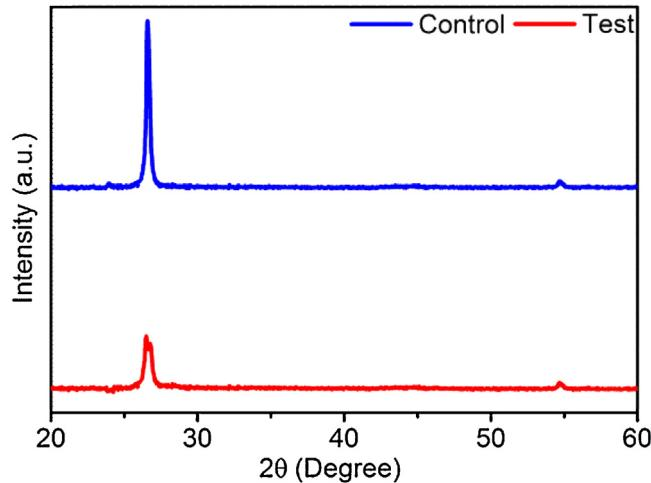
**Fig. 4.** X-ray diffraction patterns of GO samples extracted from control culture medium (in absence of bacteria) and test culture medium (in presence of resistant bacteria). The XRD pattern of test GO sample showed reduced graphitic peak intensity relative to control.
