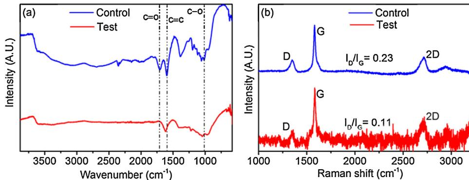
**Fig. 2.** (a) Fourier transform infrared spectra and (b) Raman spectra of graphene oxide extracted from the control (in absence of bacteria) and test (in presence of resistant bacteria) culture medium.
