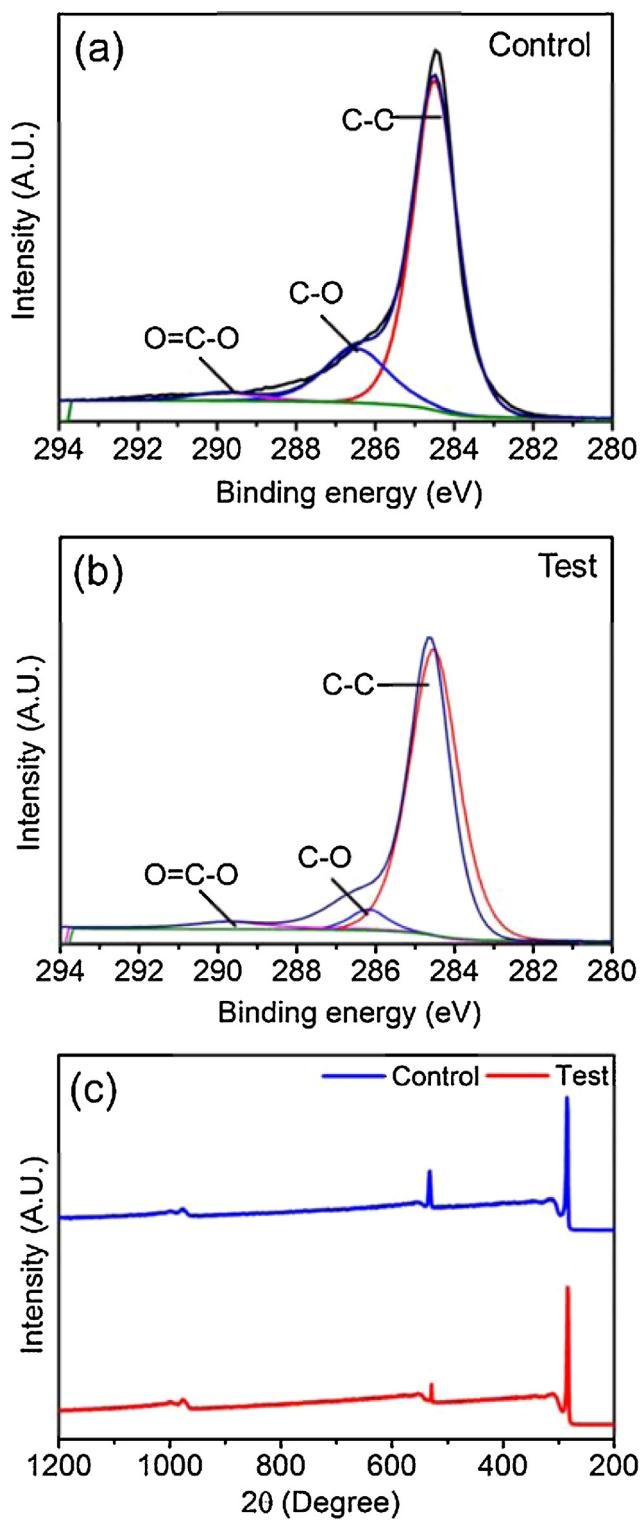
**Fig. 7.** XPS spectra of the C1s of GO extracted from; (a) control medium in absence of resistant bacteria, (b) test medium after the interaction with resistant bacteria and (c) survey spectra of both test and control GO samples.
