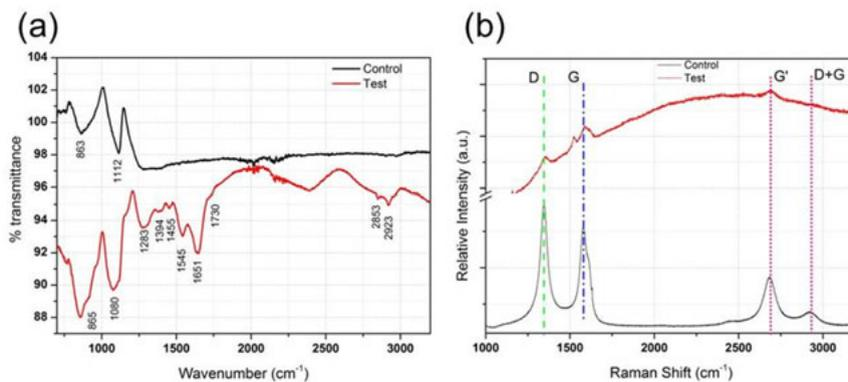
Fig. 2. (a) FTIR and (b) Raman spectra of engineered MWCNTs with and without interaction of CNTs-resistant bacteria.
