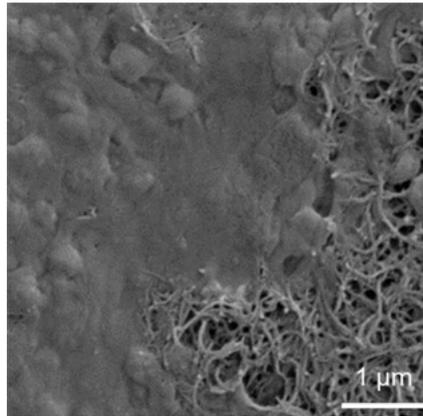
Fig. 1. SEM image showing interaction of CNTs-resistant bacteria with engineered MWCNTs.
