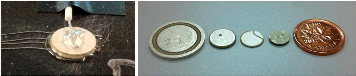
Figure 2.4: Various PZT transducers
