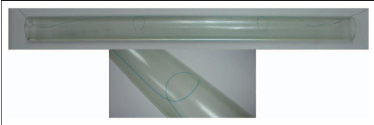
**Figure 10.** Semicircular tube with embedded fiber optic sensors.
