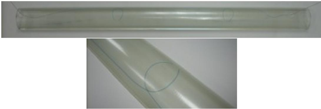
Figure 3.7: Semicircular tube with embedded fiber optic sensors
