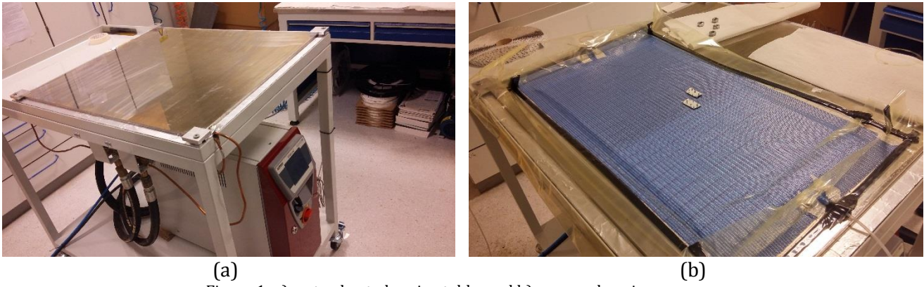
Figure 1: a) water-heated curing table, and b) vacuum bagging process
