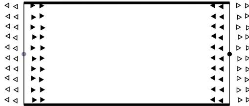
FIGURE 3.4: The sketch of the channel for which fully periodic condition is imposed in the horizontal direction. Particles denoted by  $\triangleright$  are the imaginary copies of those designated by  $\blacktriangleright$  while particles represented by  $\triangleleft$  are the imaginary copies of those shown by  $\blacktriangleleft$ .
