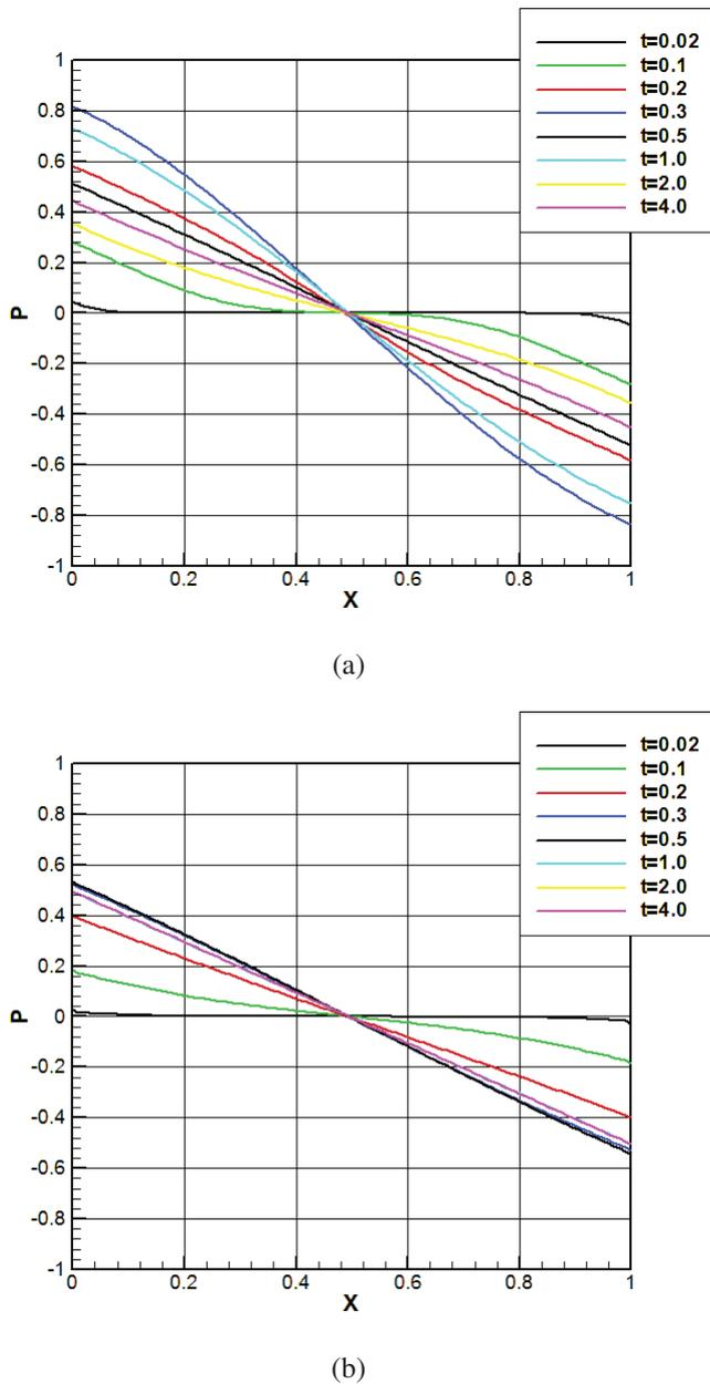
Fig. 2. Pressure results of weakly compressible SPH method of the section II-A for selected times with different viscosity coefficients; (a)  $\mu = 0.1 \text{ Pa.s}$  and (b)  $\mu = 1.0 \text{ Pa.s}$ .
