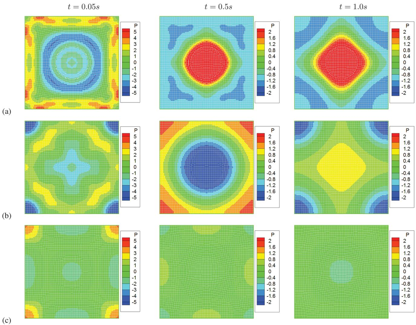
Fig. 4. Pressure distribution at different times obtained by using (a) weakly compressible with  $c=10$  m/s, (b) weakly compressible with  $c=35$  m/s, and (c) augmented Lagrangian SPH methods.
