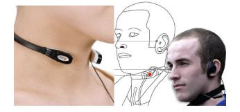
**Figure 1.** Conceptual designs for the proposed wearable mobile device using SSI together with auditory feedback
